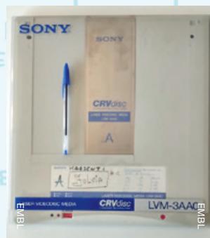
Write once, read many – these CRV discs were used largely as early portable data backups.
